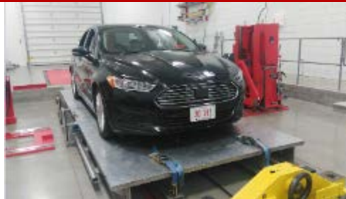
Vehicle Inertia Parameters Test
