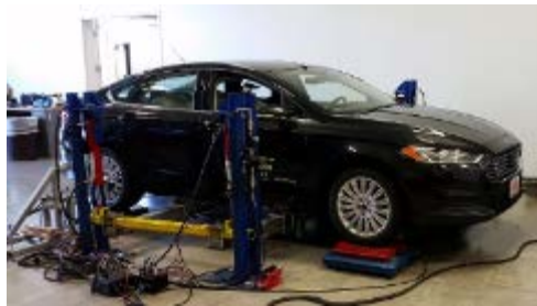
Suspension Kinematics & Compliance Test
